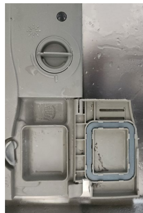
The detergent loading part of my dishwasher. The top part is for pre-rinse, the middle is pre-wash, and the bottom part is the actual detergent location.
